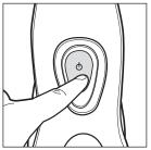
Press ON/OFF button. Wait 20 seconds for unit to heat up. Unit may vibrate while heating.
